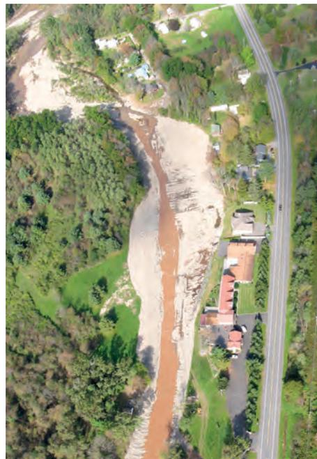
Stream channels in the Catskills are sometimes excavated and reshaped to protect infrastructure or reduce flooding. If not done with sufficient knowledge, channel modifications can easily affect sediment transport and trigger channel erosion near roads, bridges, homes, or businesses.
