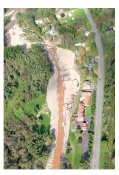
Stream channels in the Catskills are sometimes excavated and reshaped to protect infrastructure or reduce flooding. If not done with sufficient knowledge, channel modifications can easily affect sediment transport and trigger channel erosion near roads, bridges, homes, or businesses.
