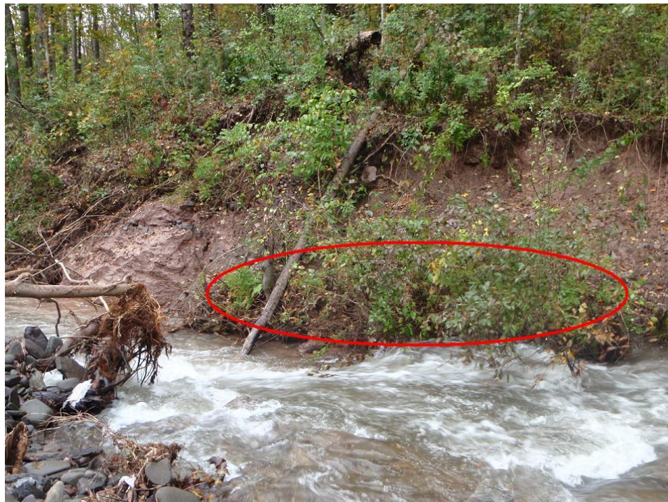
Figure 10: High erosive variability was observed in this type of non-alluvial boundary condition. Decreased shear strength after saturation from storms and removal of toe support initiated this geotechnical failure that created a shelf exposed below bankfull elevation. The red circle illustrates the section of vegetated-glaciolacustrine clay layer that slumped near the water surface.
