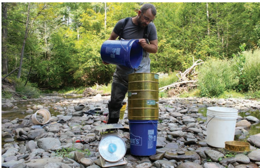
Sediment sampling at one of two Warner Creek stream restoration sites slated for construction in 2021. Extensive survey, design and engineering were completed to prepare for construction.
