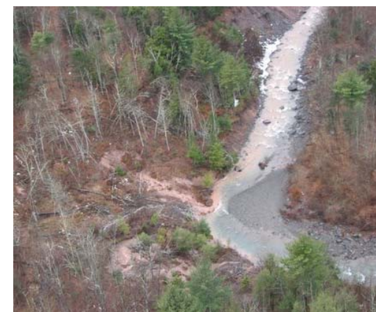
Turbid ground water seeps out of hill slope failures into the Stony Clove
