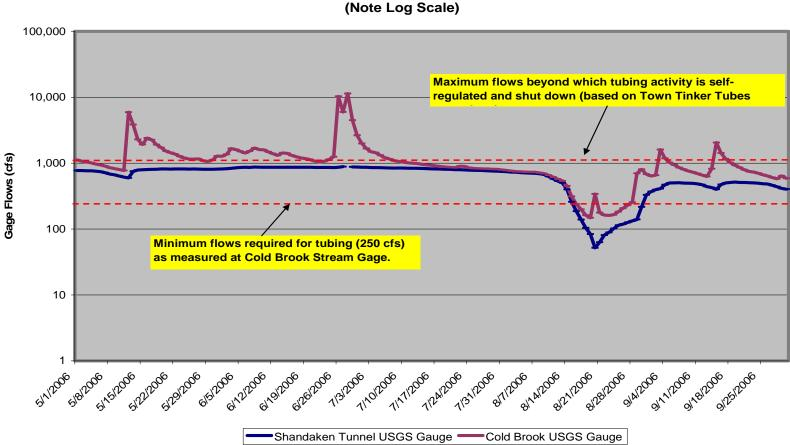
Stream Flow and Shandaken Tunnel Discharge Data Mean Daily Values: May 1 - September 30, 2006 (Note Log Scale)
