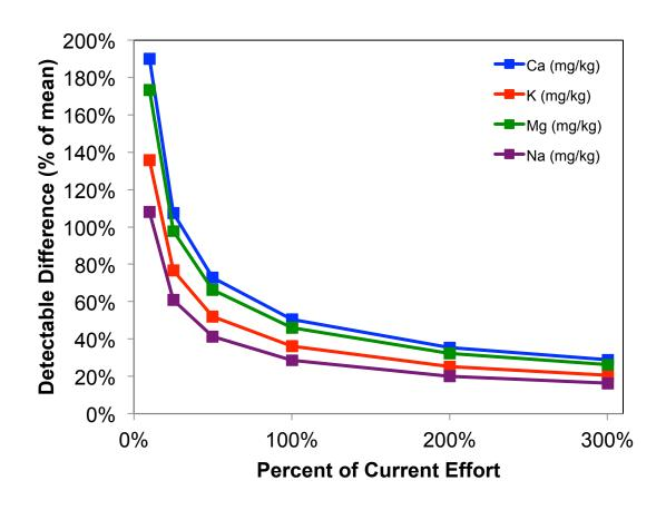
These case studies illustrate the effect of sampling intensity on statistical power and the selection of a sampling interval likely to detect an expected change over time
