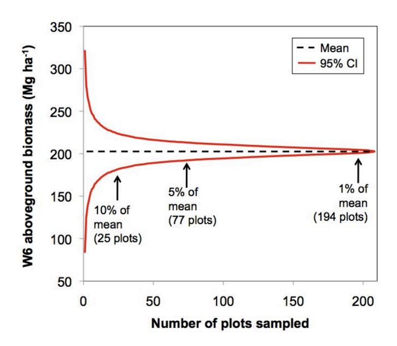
Yanai et al. (2010, Ecosystems) estimated uncertainty in the Hubbard Brook Valley, including measurement error of tree diameters, uncertainty in allometric equations, and sampling error (with varying numbers of plots)
