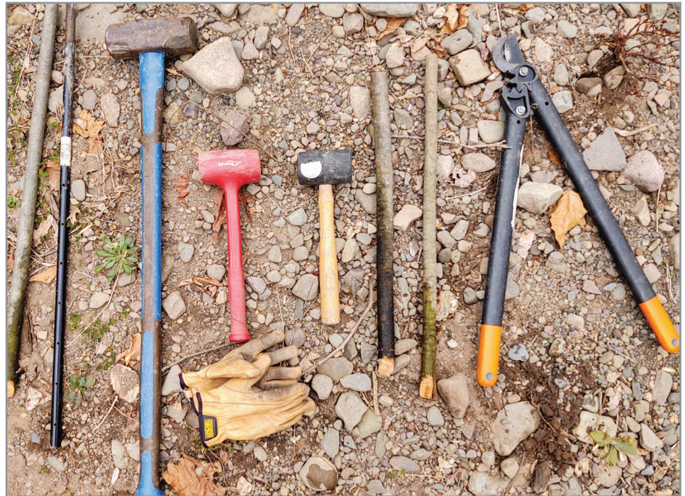
Required tools, from left to right: willow stake, concrete form pin, sledgehammer, dead-blow hammer, work gloves, rubber mallet, willow stakes, loppers.
