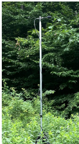
A bat acoustic survey array basically looks like a mic on a stand near a stream. A biologist will review the captured sound for the presence of the endangered Northern long-eared bat. If detected, tree clearing for stream projects will be delayed to avoid harming the now-rare bats.
